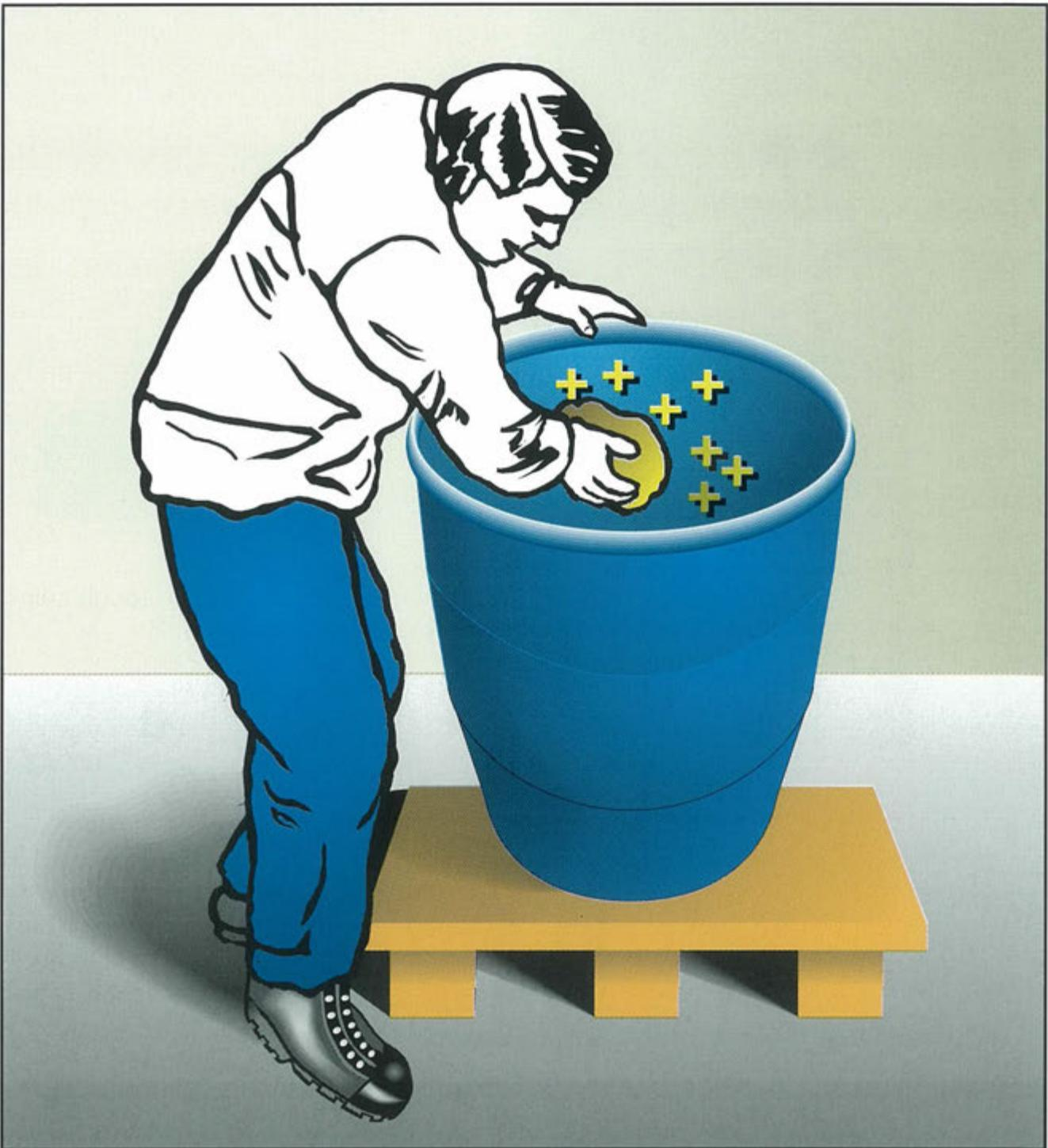
Fig. 35: Formation of high charges through friction (secondary processes)
