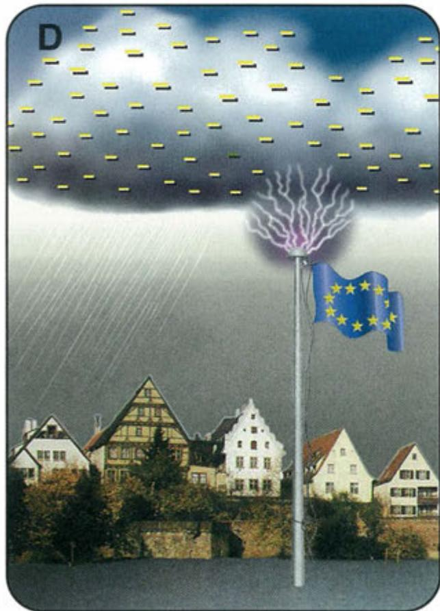
Fig. 23: Examples of brush discharges in practice – A: through charged bulk material container B: through charged insulating liquid C: through charged dust cloud D: through charged storm cloud
