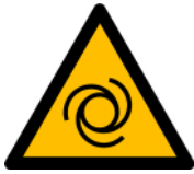
Figure 3: “Unexpected start-up” warning sign on the cover of contactors
