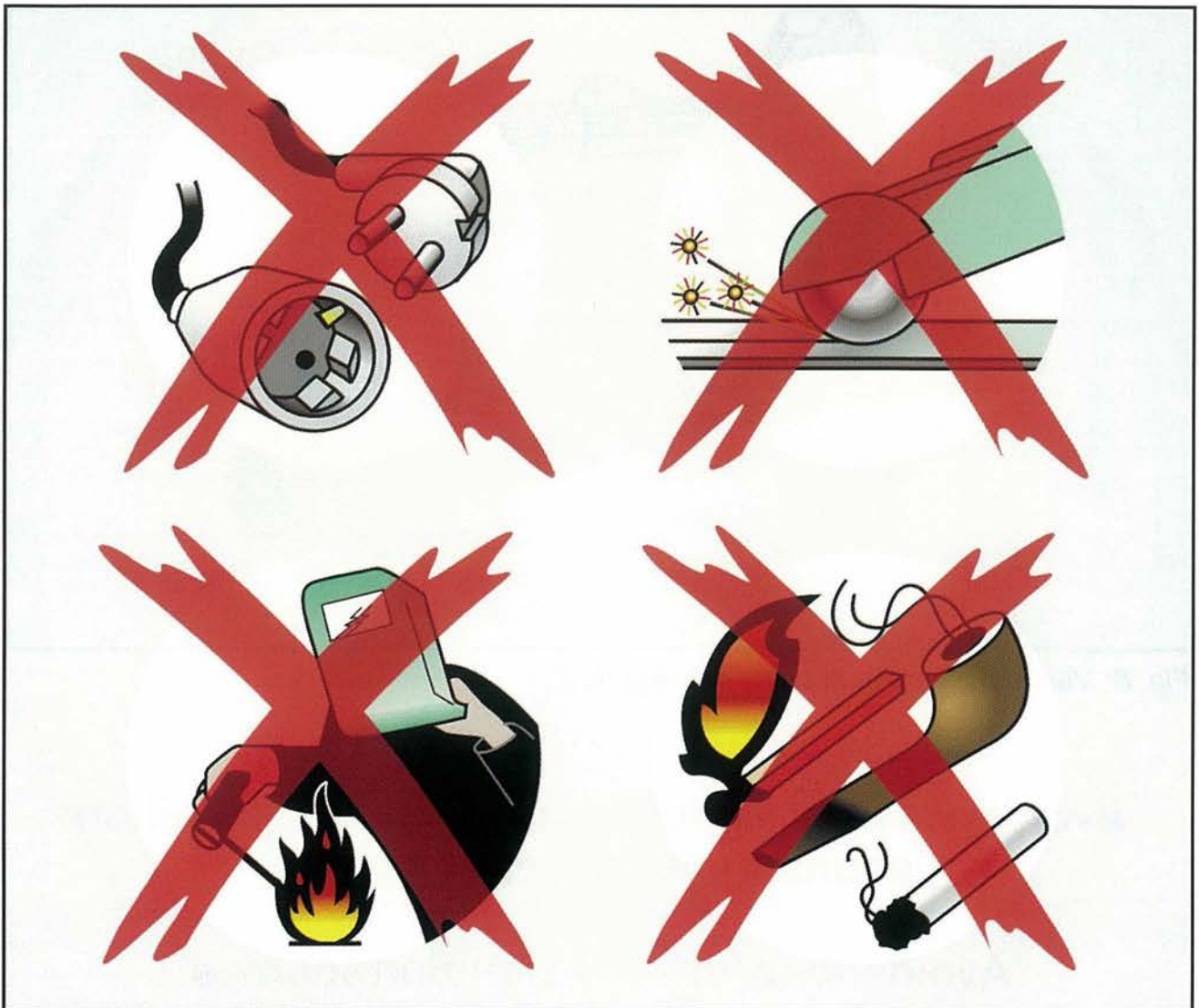
Fig. 7: Avoidance of effective ignition sources
