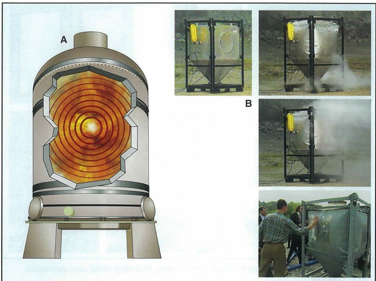
Fig. 10: Examples of explosion pressure resistant vessels.
