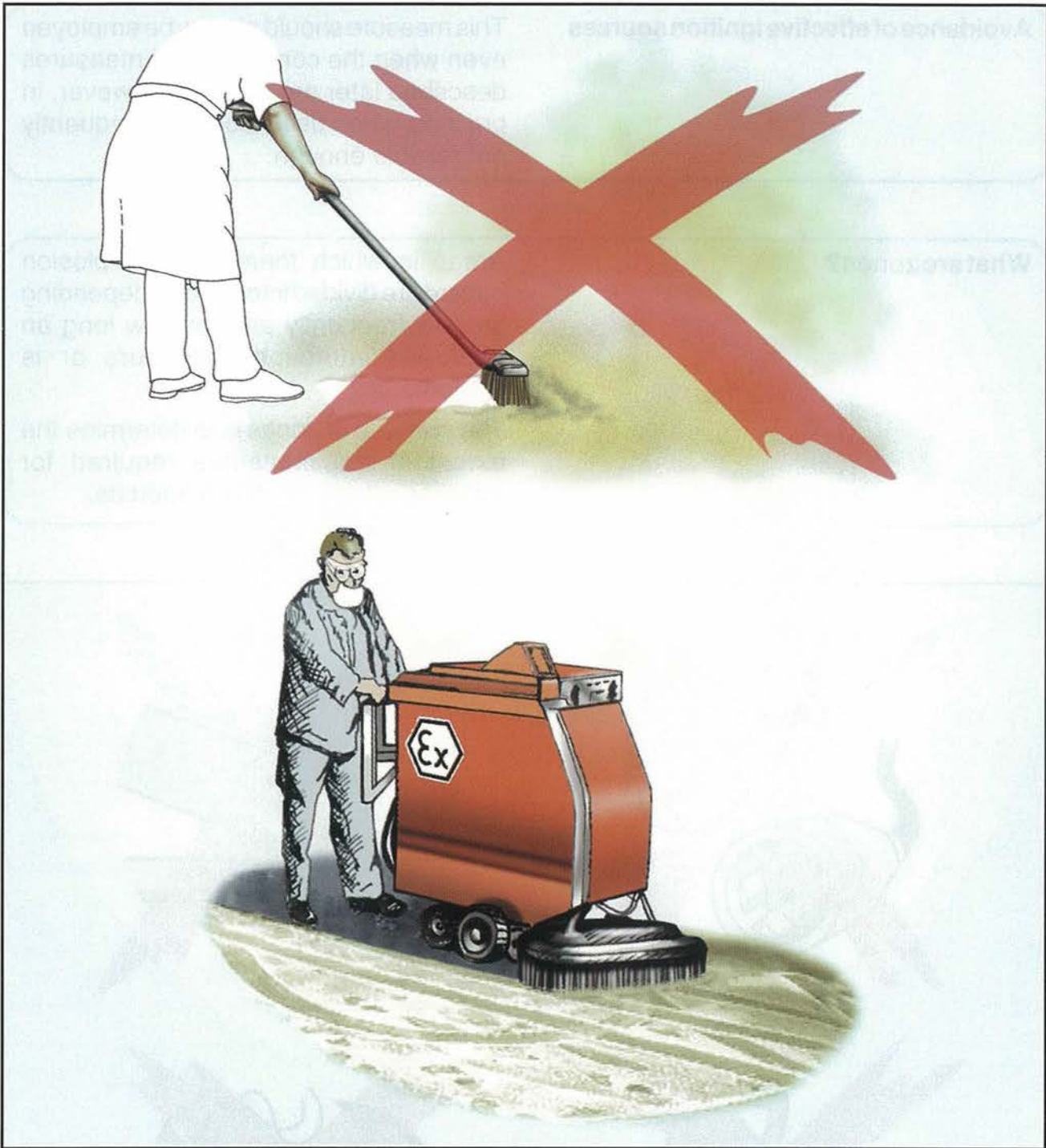
Fig. 8: Vacuum cleaning to avoid blowing dust
