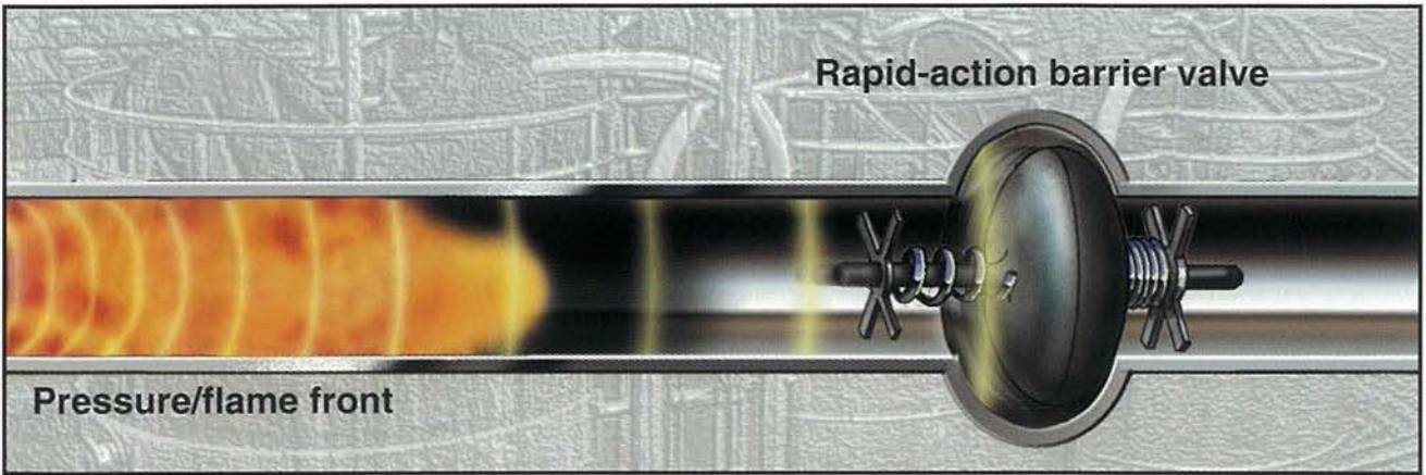
Fig. 17: Explosion isolation by rapid-action barrier valve
