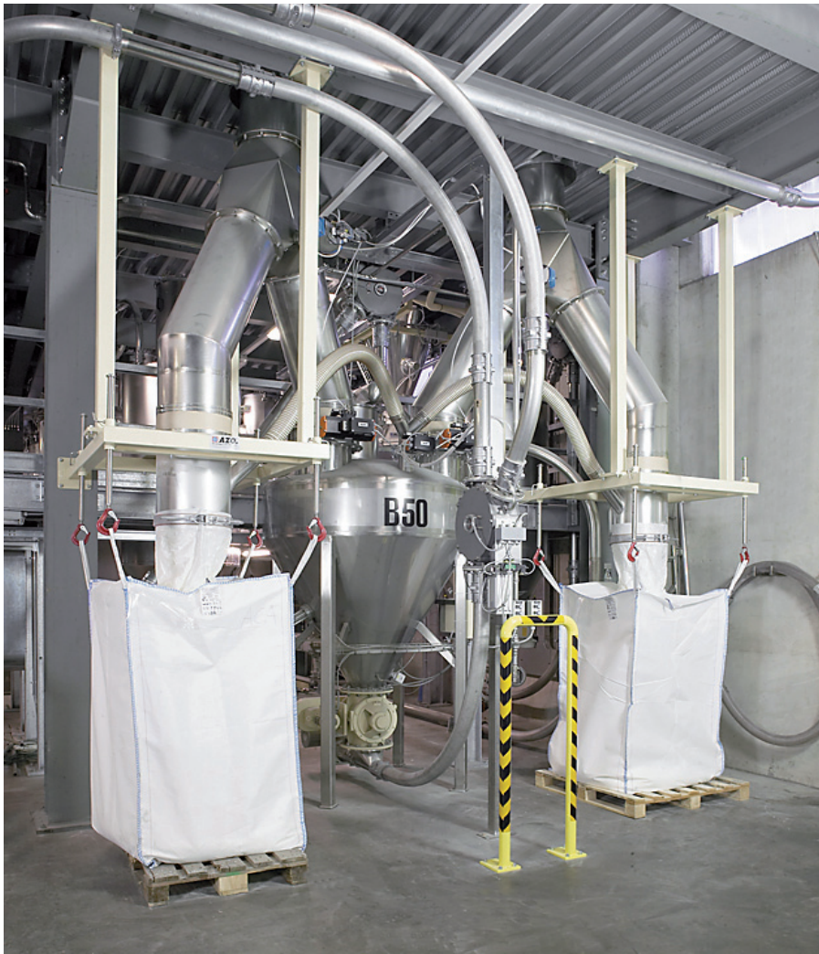
Figure 18: FIBC filling (Source: AZO® GmbH + Co. KG)
