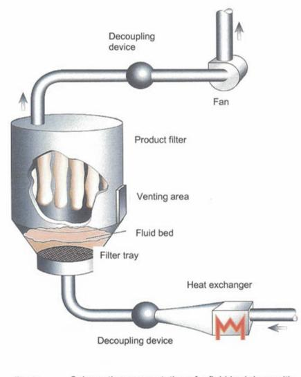
Fig. 2: Schematic representation of a fluid bed dryer with protection by explosion venting
