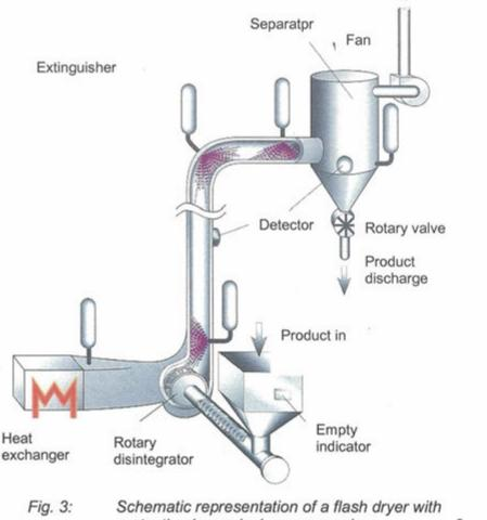
The product is exposed to fairly low and short-term thermal stress in spite of high air inlet temperatures (evaporation heat). If product deposits and caking are formed on the wall or ceiling of the dryer, the assessment of thermal stress of a product must take into account a long-term stress which can rapidly lead to ignition, in particular in the area of the high inlet temperatures. This can result in a dust fire or - in particular in case of dropping smoldering lumps - in a dust explosion.
