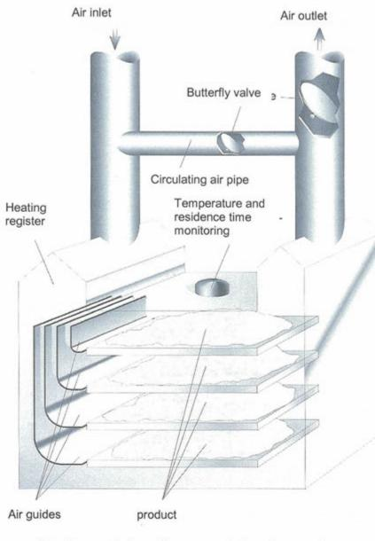
Fig. 8: Schematic representation of a pan dryer
