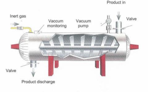
Fig. 7: Schematic representation of a vacuum paddle drye
