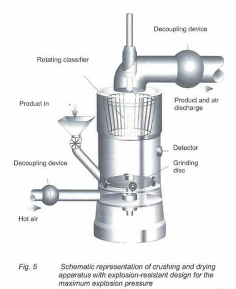
In addition to the thermal stress, the products are simultaneously exposed to mechanical stress caused by the crushing process. Additional mechanical stress can be caused by dynamic classifiers integrated in the mill. The relative speeds of the moving parts are considerably higher than 1 m/s. In particular in cases when tramp matter is introduced or failures occur, mechanically generated sparks or hot surfaces cannot be ruled out. These may ignite both dispersed and deposited dust.
