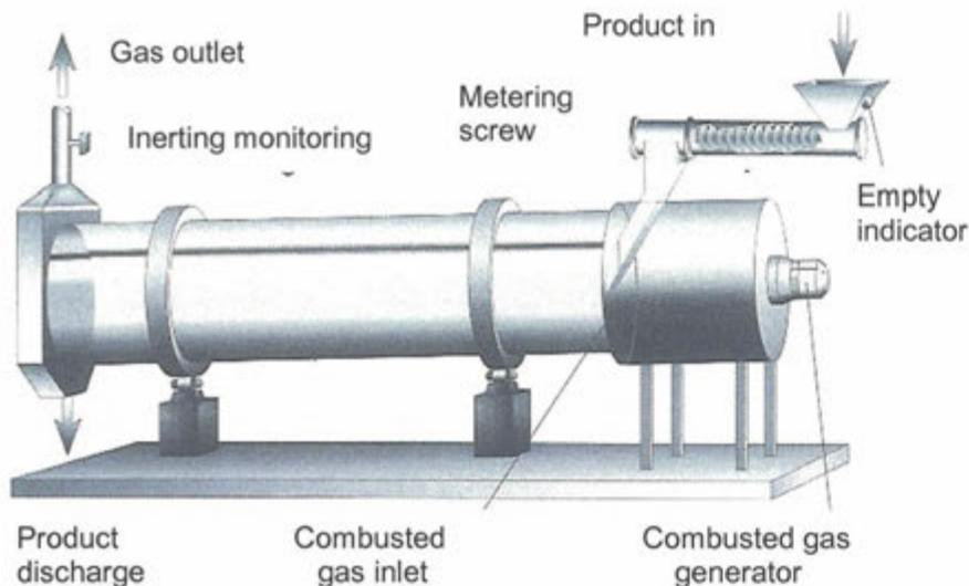
Fig. 6: Schematic representation of a drum dryer with inerting using combusted gas
