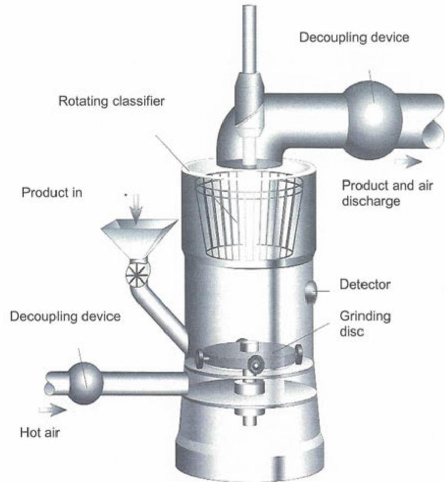
Fig. 5 Schematic representation of crushing and drying apparatus with explosion-resistant design for the maximum explosion pressure
