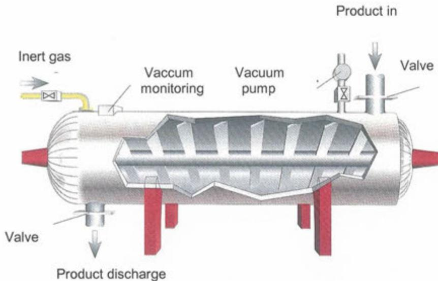
Fig. 7: Schematic representation of a vacuum paddle dryer
