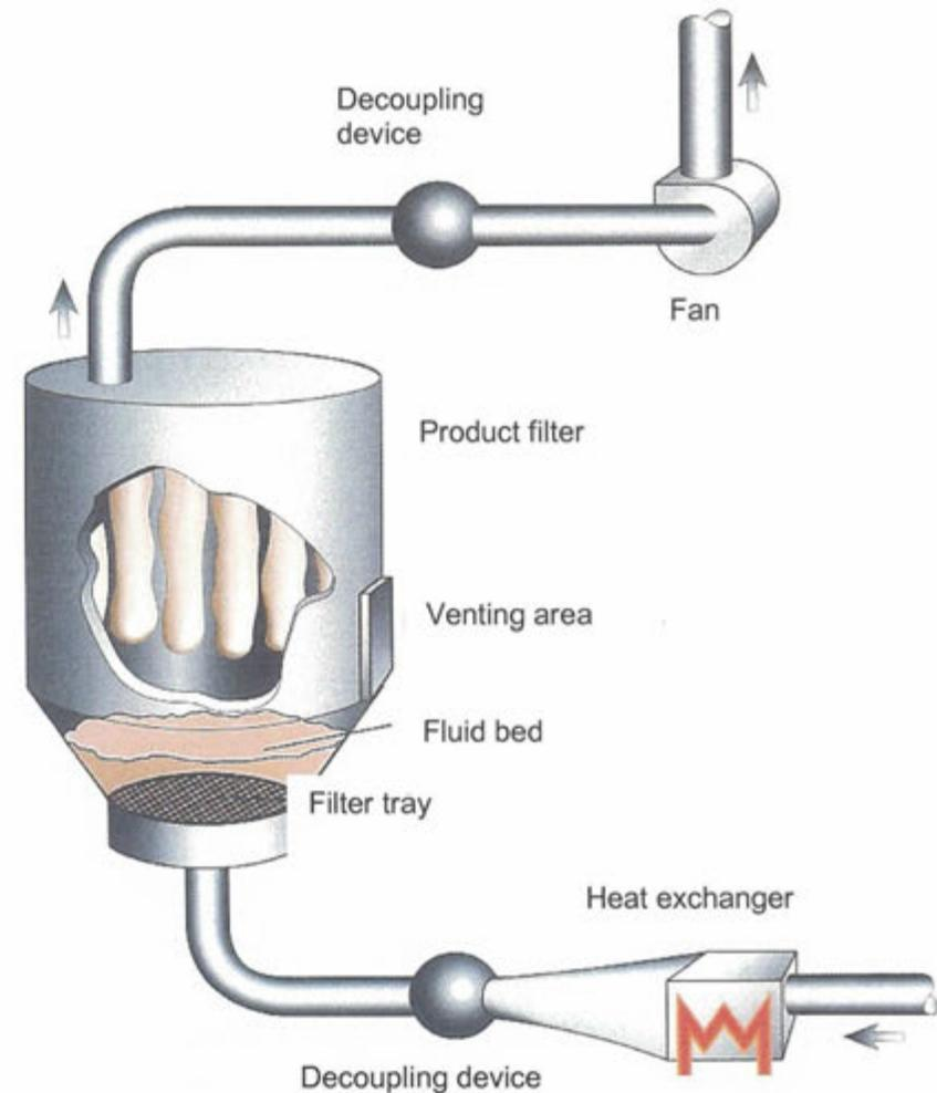
Fig. 2: Schematic representation of a fluid bed dryer with protection by explosion venting
