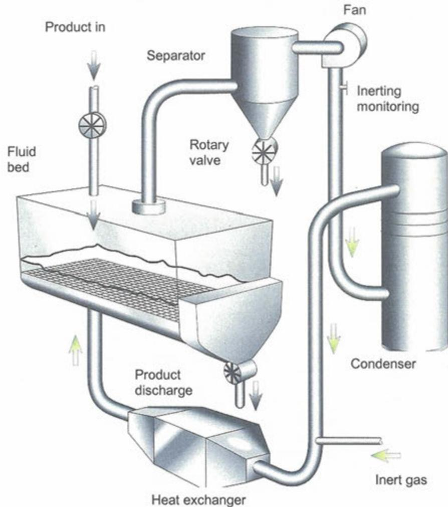
Fig. 4: Schematic representation of a fluidized bed dryer with protection by inerting (closed circulating system)
