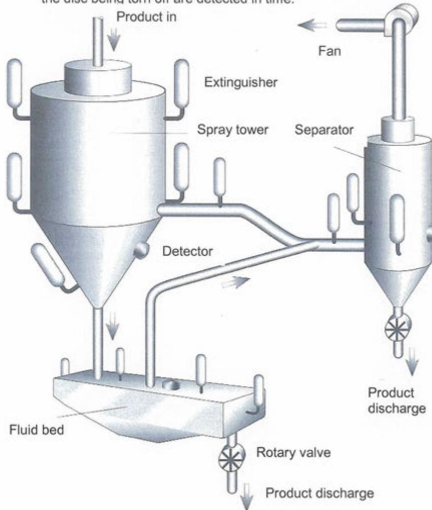
Fig. 1: Schematic representation of a spray dryer system protected by explosion suppression measures
