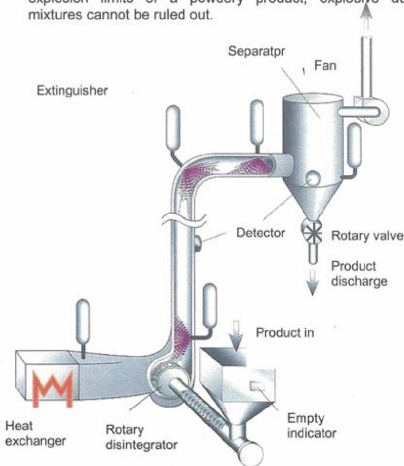
Fig. 3: Schematic representation of a flash dryer with protection by explosion suppression
