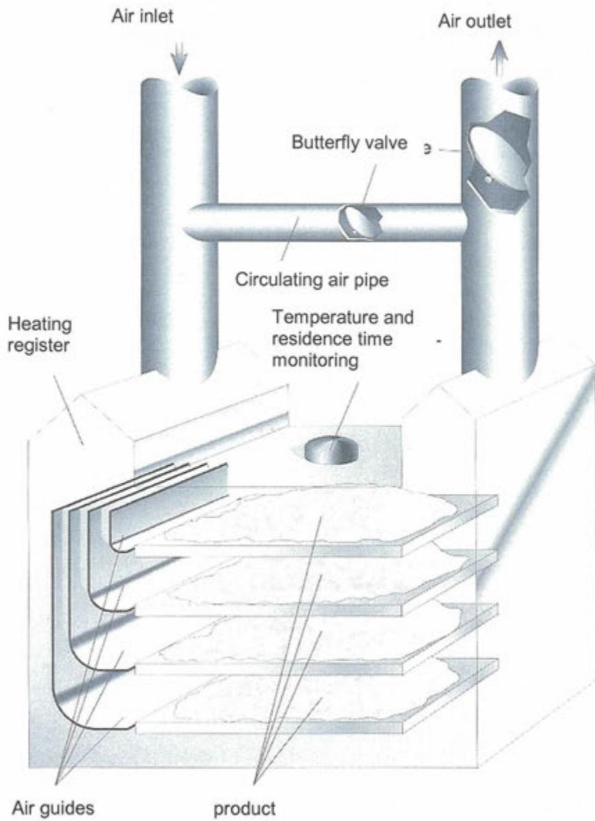
Fig. 8: Schematic representation of a pan dryer
