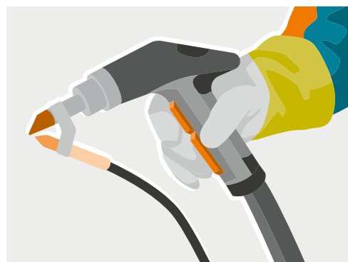
2 Laser welding gun with two-button activation
