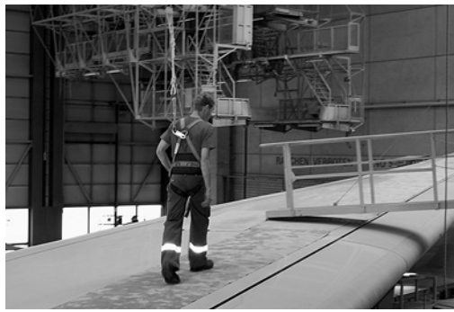
7 Fall protection when leaving a working platform.
