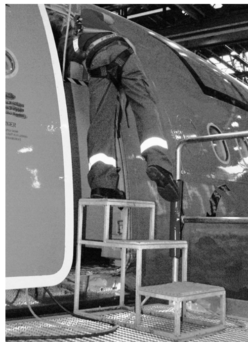
6 Fall protection when using a triple-tread step.
