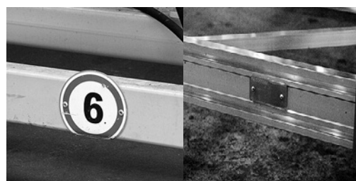
4 Maximum speed is clearly marked. Reflector for enhanced visibility in the dark.
