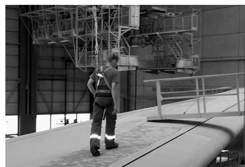
7 Fall protection when leaving a working platform.
