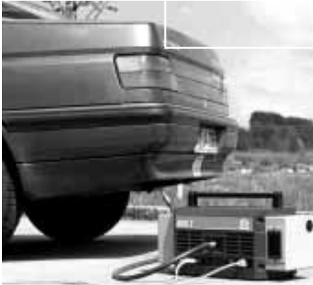
Fig. 7: Regular checks are made using an opacity meter (being used here on this diesel car) to see whether the PFS is satisfying the required rate of separation.
