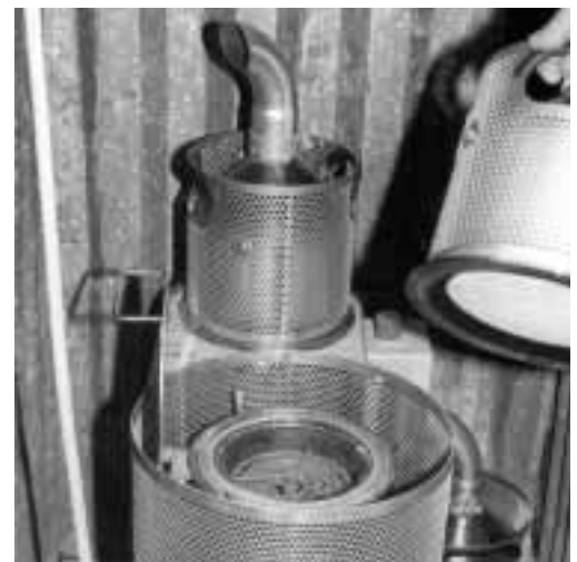
Fig. 2: Burning-off station for the regeneration of replaceable PFS.
