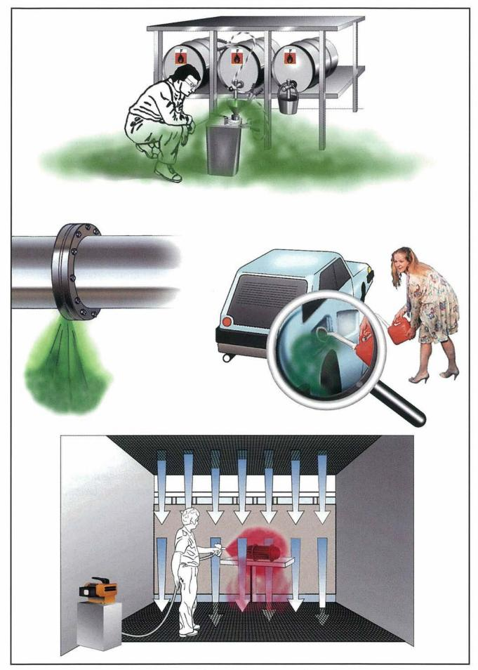
Fig. 1: Examples of the formation of vapors and mists from flammable liquids
