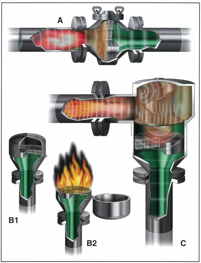
Fig. 12: Explosion isolation by
