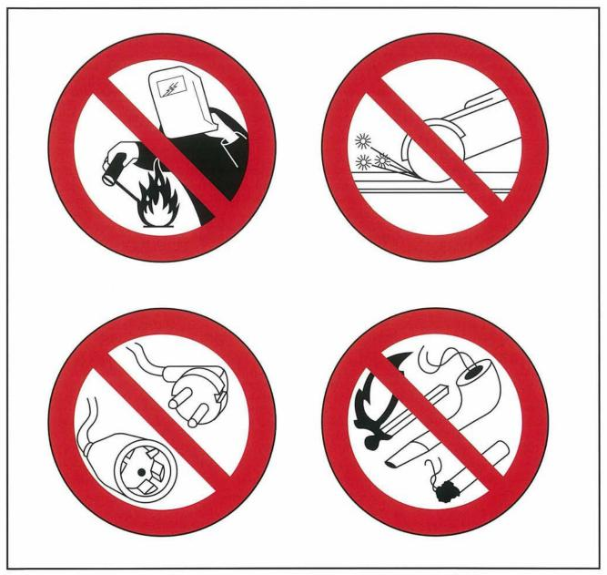
Fig. 9: Avoidance of effective ignition sources
