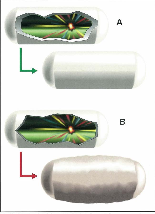
Fig. 11: Examples of explosion-resistant tanks before and after occurrence of an explosion - A: explosion-pressure-resistant construction B: explosion-pressure-shock resistant construction
