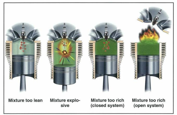
Fig. 4: Explosion limits
