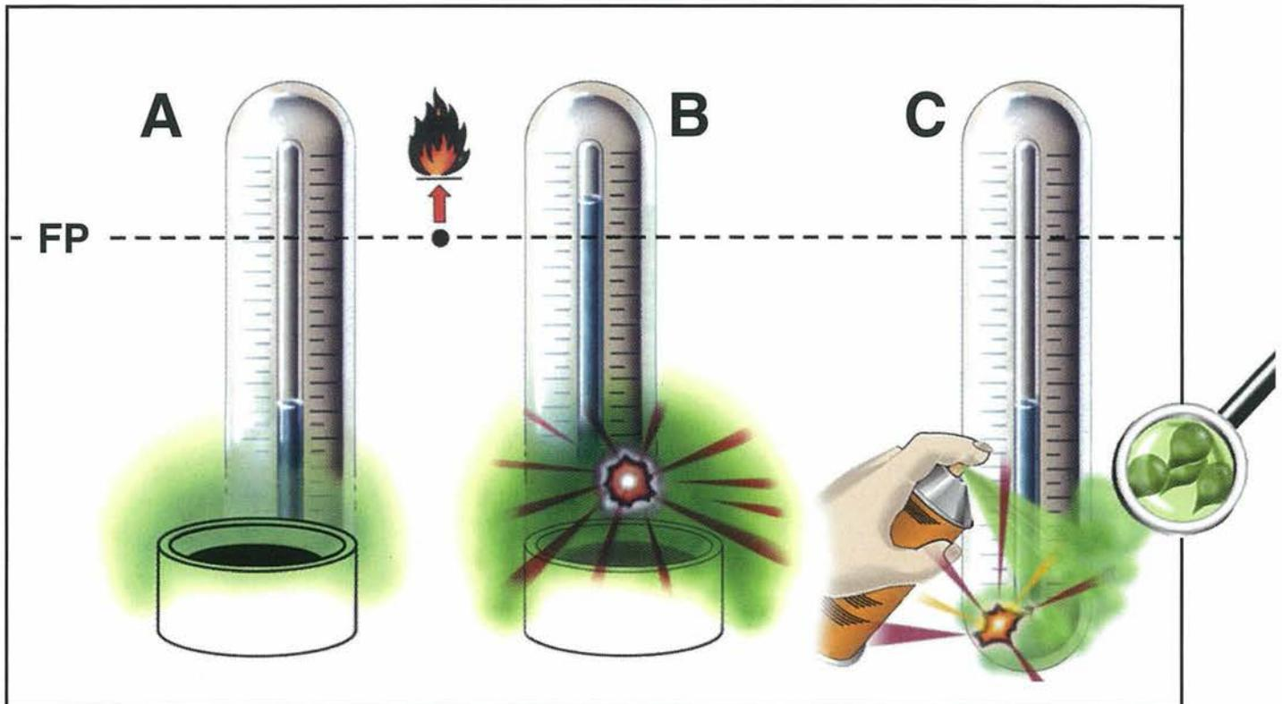
Fig. 2: Illustration of the flash point (FP)
