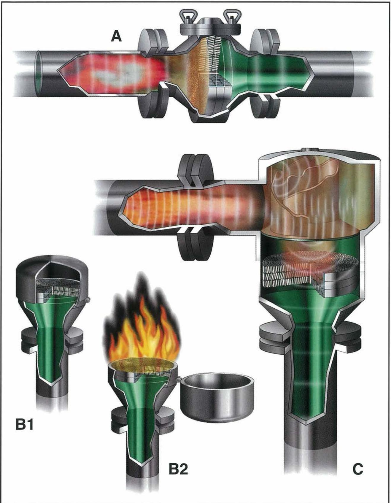
Fig. 12: Explosion isolation by
