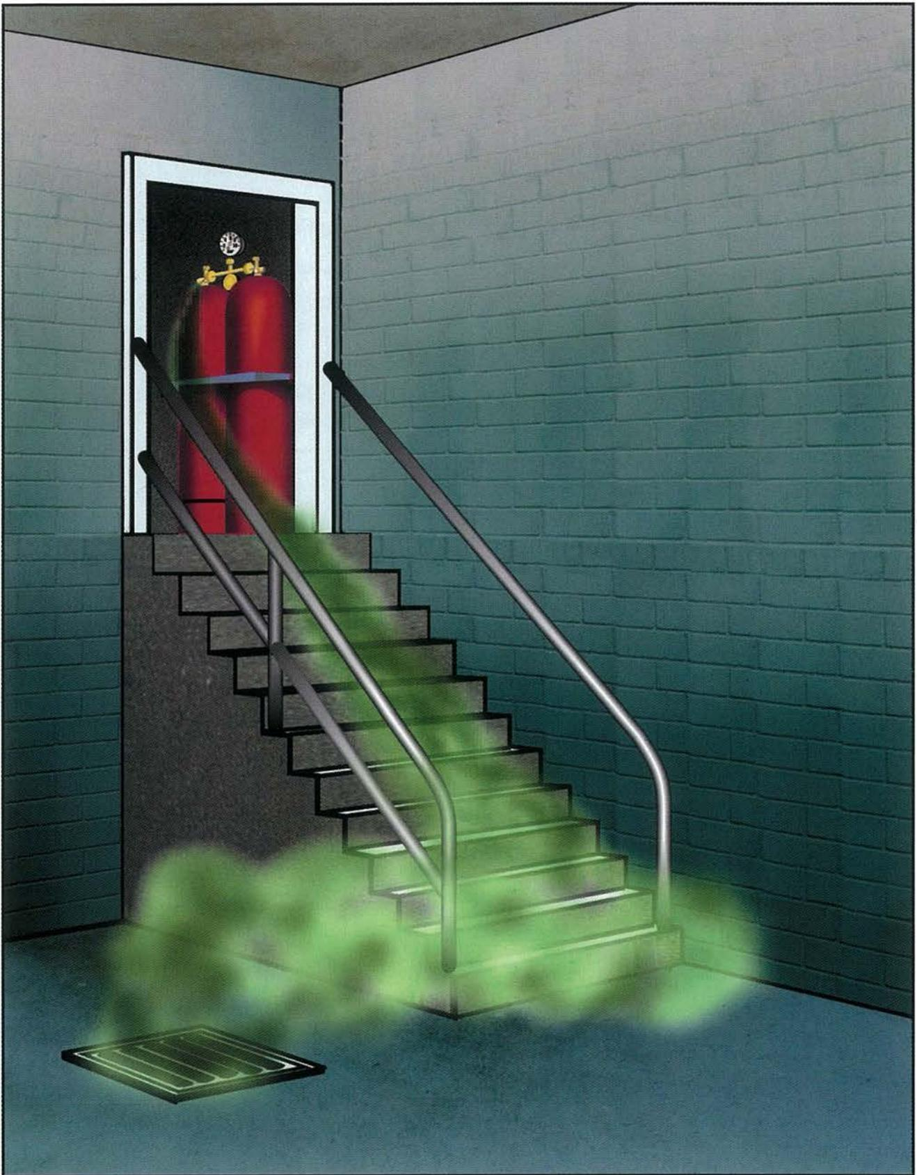
*Fig. 6: The spreading behavior of liquified gas (taken as example)*
