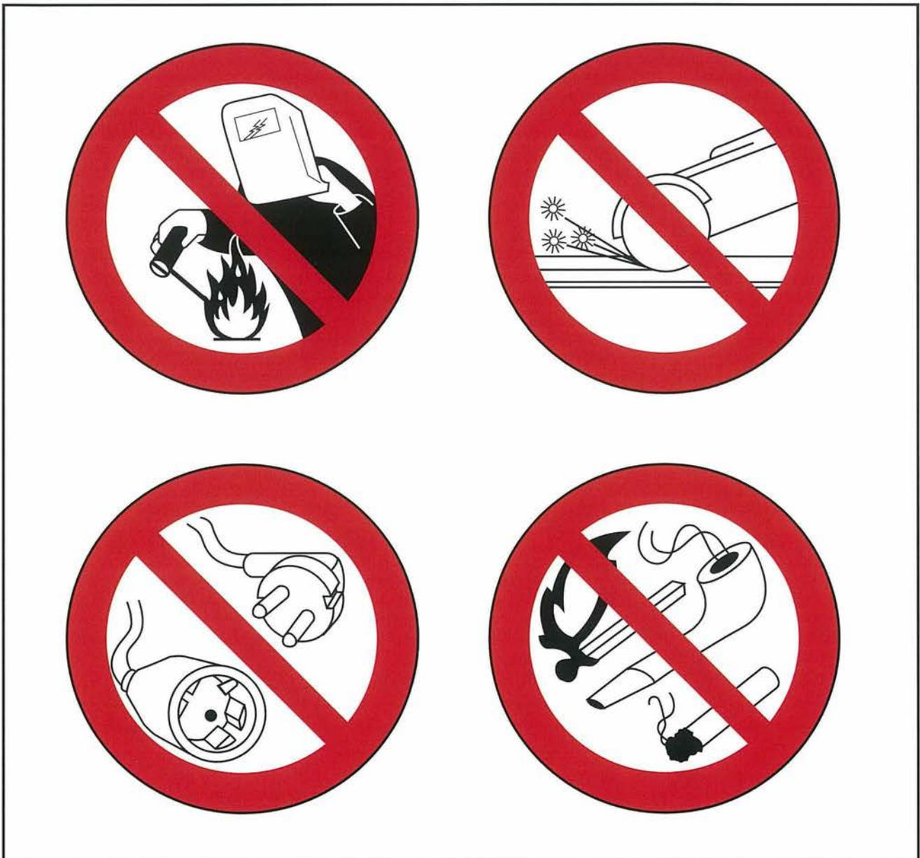
Fig. 9: Avoidance of effective ignition sources
