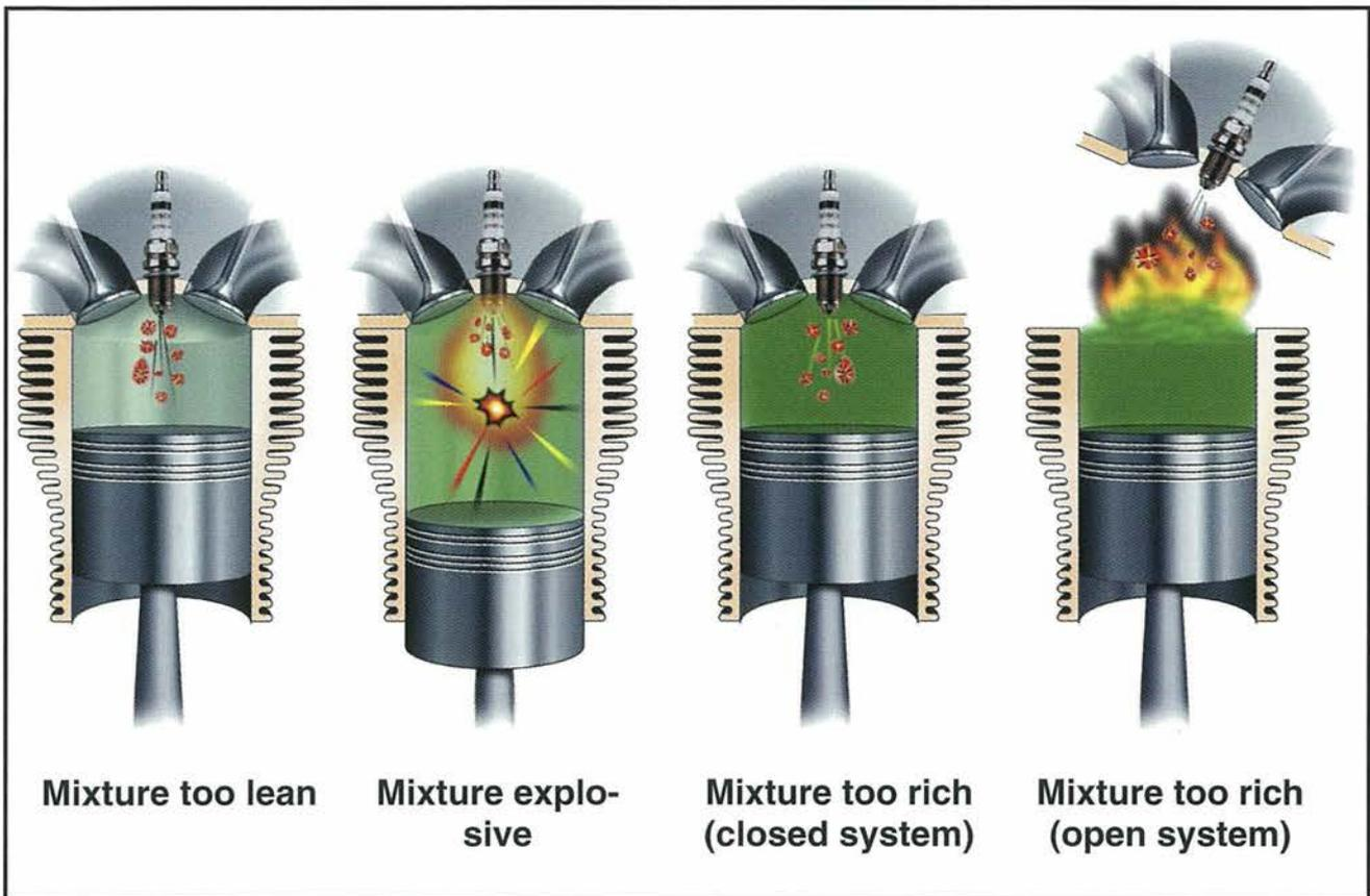
Fig. 4: Explosion limits
