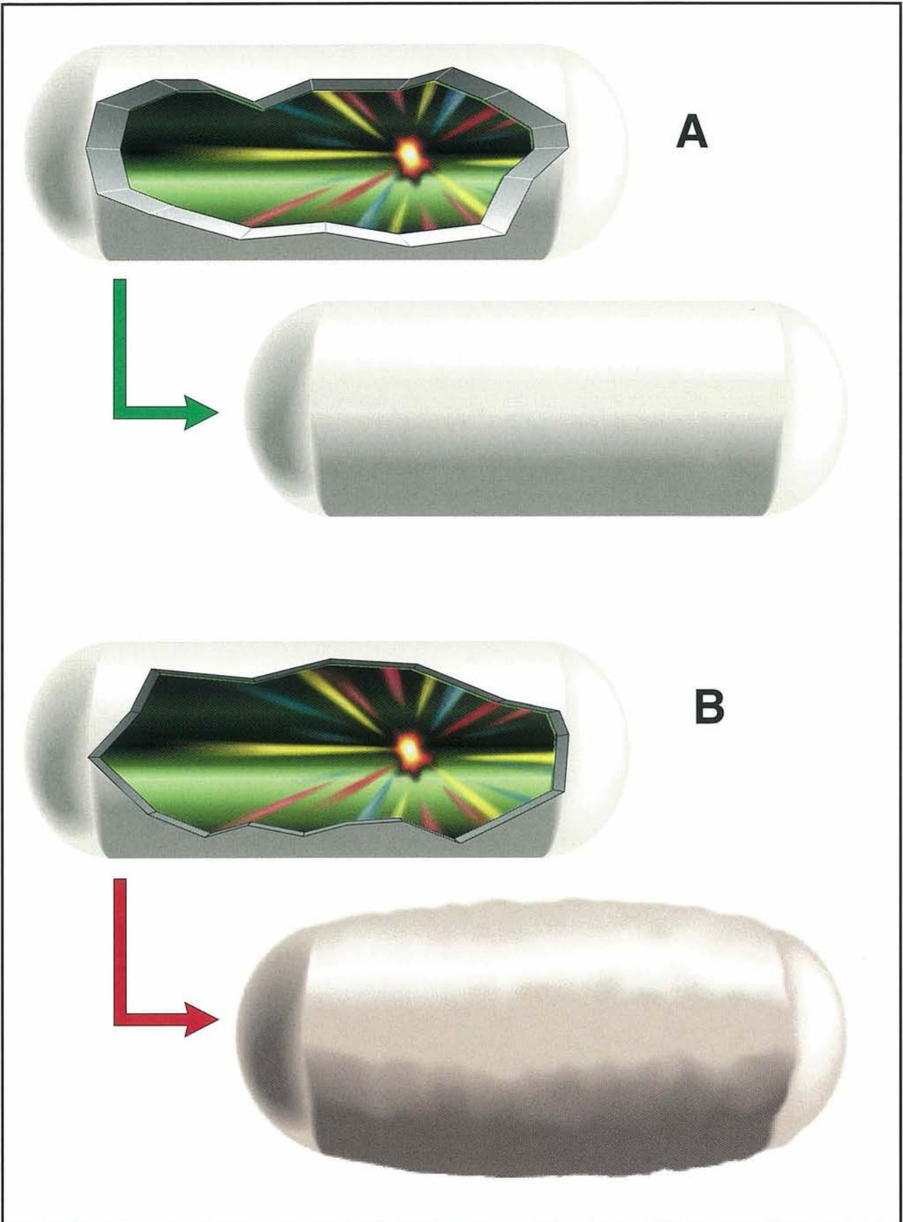
Fig. 11: Examples of explosion-resistant tanks before and after occurrence of an explosion - A: explosion-pressure-resistant construction
