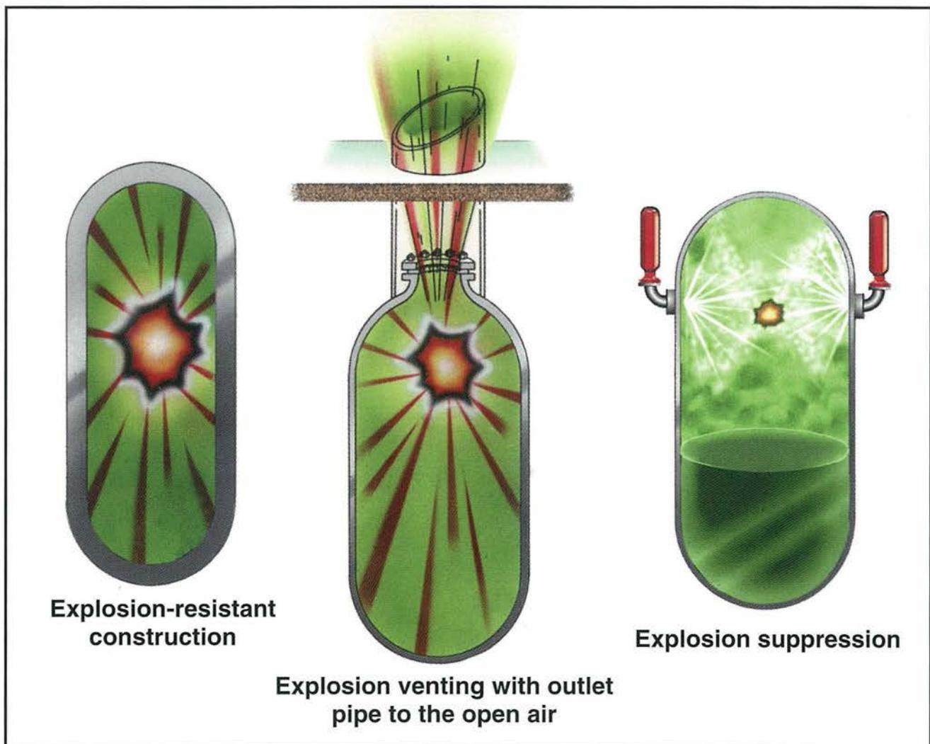
Fig. 10: Examples of constructional explosion protection measures
